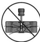
This icon warns you to not over tighten your bolts. This is to prevent structural damage and also splintering your wood.
