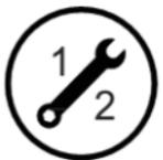
This icon shows the size of an open ended wrench. Using the wrench as the fraction bar.
