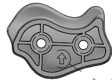
**NOTE: FOR PROPER ASSEMBLY ARROW POINTS TO THE TOP OF THE ROCK.**
